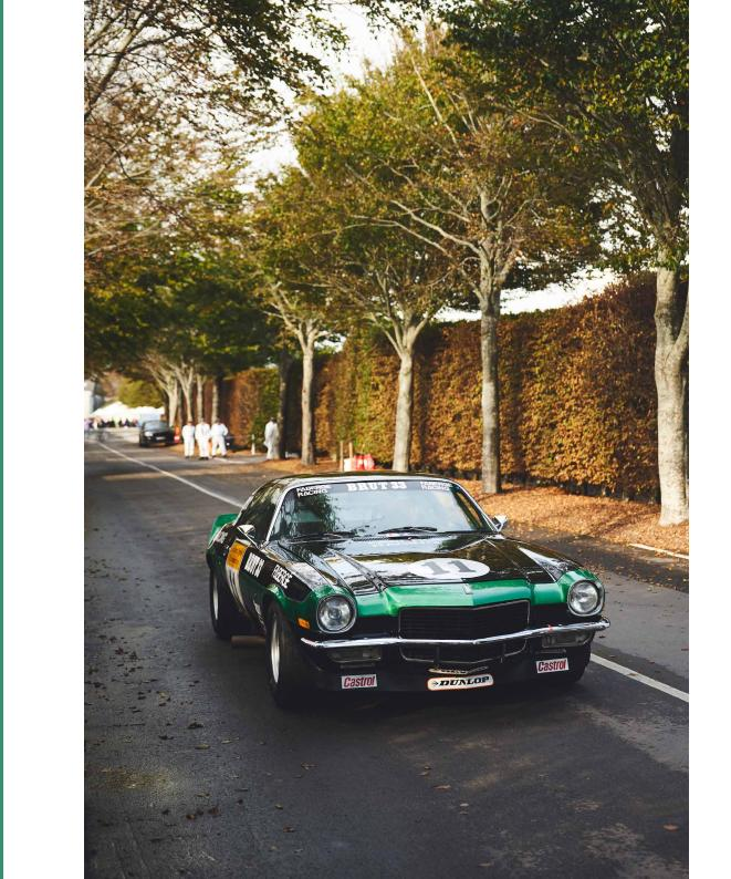
The car has a fresh Pete Knight engine, the T-10 close ratio direct top Road Race Spec gearbox has new synchros and the belts, extinguisher, etc are in-date. Spares include: 2nd set of 4 wheels and tyres, new BG Developments front discs and bells, front brake calipers and bedded pads.
