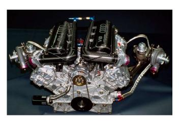
What was carried over from the R8R and R8C was the powerful but frugal twin-turbo V8, designed inhouse by Ulrich Baretzky. Constructed from lightweight aluminium-alloy, the compact engine displaced just under 3.6 litres and was equipped with a pair of Garrett turbochargers. Once fitted with the mandatory restrictors, the V8 initially produced around 600 bhp. The engine was mated to a Ricardo-sourced six-speed sequential gearbox, which was operated by steering wheel mounted paddles.
