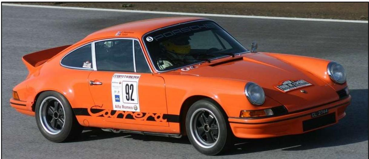
To save weight the M471 was fitted with thinner steel body panels, glassfibre replaced some and thinner window glass. The interior was stripped, soundproofing was removed, flat door panels were used with a strap to
