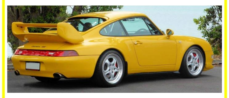
The 993RS follows the same path as the earlier 911RS in being a lighter and more powerful variant of an already extremely capable sports car. 100 Kgs lighter and with a 300bhp 3.8 litre engine, improved aerodynamics and bespoke "Speedline for Porsche" 18" modular wheels.
