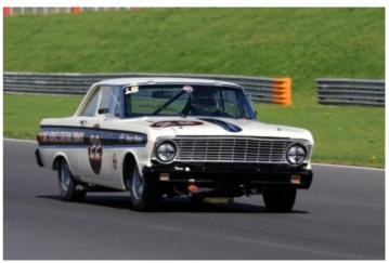
This Falcon was purchased from Stefano Rosina in Italy where it had been a successful FIA race car. The shell was completely stripped and the car rebuilt in early 2018 and is in immaculate condition with fibreglass boot, doors, wings and bonnet, polycarbonate side and rear windows, it weighs 1,158kg.
